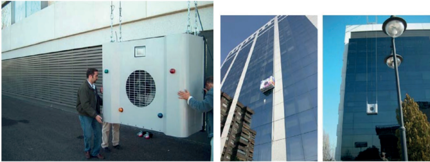
Figure 8. Tito 500 façade cleaning robot (Akinfiev et al., 2009)
