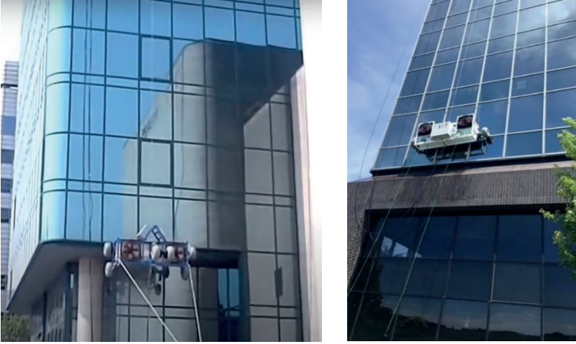
Figure 9. Sky Pro façade cleaning robot (URL-9)
