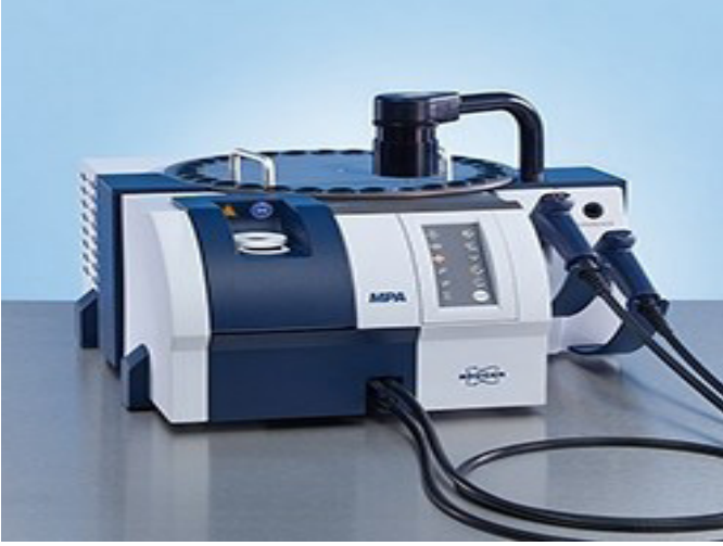
Picture 3. An NIR device used in feed analysis
