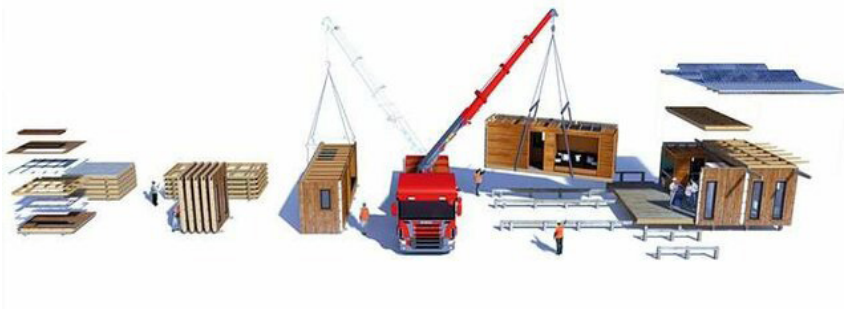
Figure 8. Production Process of Prefabricated Buildings (Patwari, 2020)
