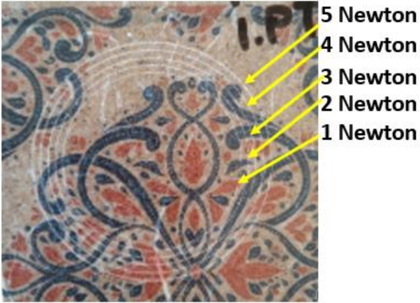
Figure 4. Worse sample (I2) Scratch circles
