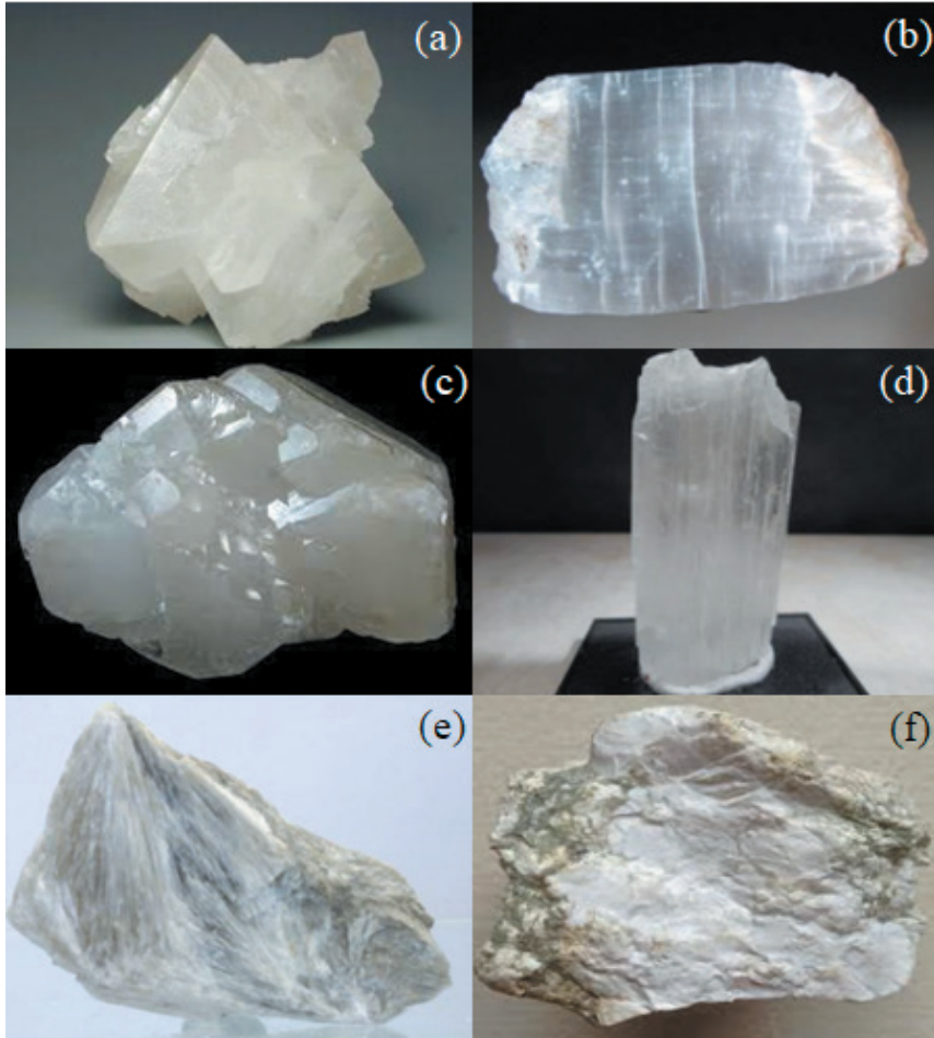
Figure 2. Boron containing minerals (a) Borax (Tincal), (b) Ulexite, (c) Colemanite, (d) Kernite, (e) Probertite, (f) Pandermite [7, 8]
