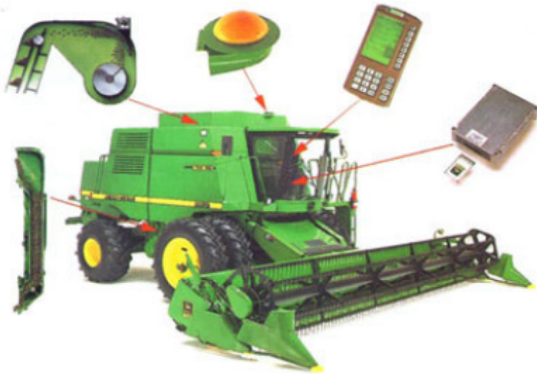
Figure 4. Parts of a consolidate mounted yield-observing framework. Clockwise from left, Movement sensor, yield screen, worldwide situating framework, yield-screen show, and information recording gadget. (Morgan, & Ess, 1997).
